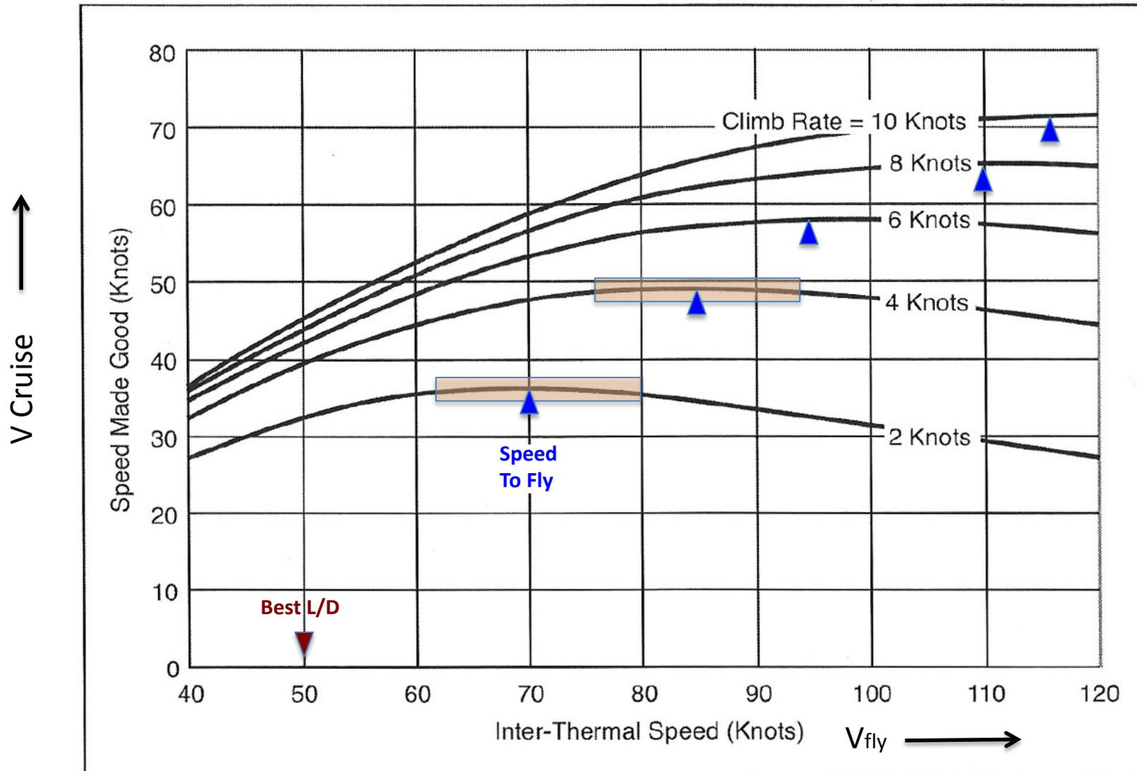
Figure 15.12 – The speed-to-fly for a given climb rate is indicated by the peak of the curve. For example, the speed-to-fly for a 4-knot climb rate is 85 knots. (These curves are for a Duo Discus at 6.2 pounds per square foot wing loading, with a best L/D of 45:1 at 50 knots.)
