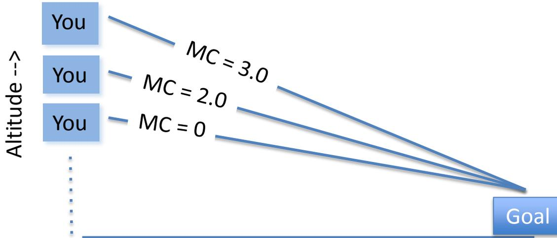
Note especially that a higher MC value dictates a higher average sink rate over the glide. This sink can come from your speed or sinking air (usually a combination of both)
