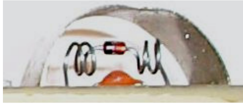
Figure 2 - Thermal Snooper sensing silicone diode
